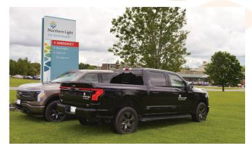
which typically takes up a lot of space". The trucks are efficient in battery use, and after being charged overnight, they will last all day with a range of up to 240 miles. There are no fuel or oil change costs, and since AR Gould is connected to the Canadian electric grid, any electricity used to charge the vehicles is sourced from hydro and nuclear plants.
